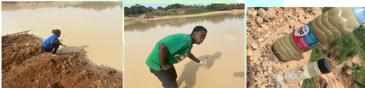
Figure 3. 6: Picking of water samples (and later preserved with HNO_3 ) to be transported for analysis
