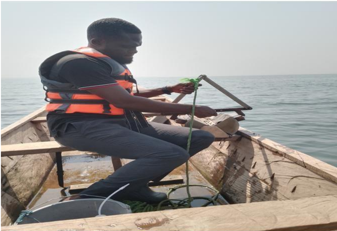
Sediment sampling with van Veen grab at Kpebe
